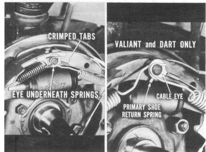
Fig. 18 — Install cable eye correctly
