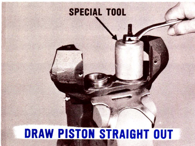
Fig. 3—Piston cocking can cause damage
