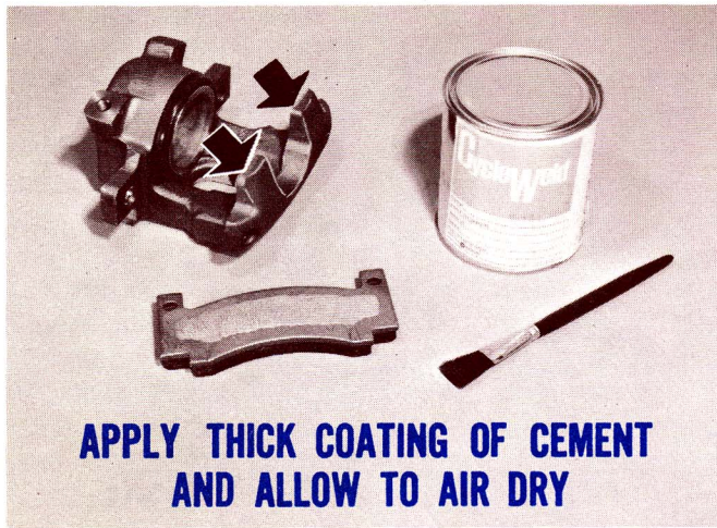
Fig. 14—Coat shoe and caliper surfaces
