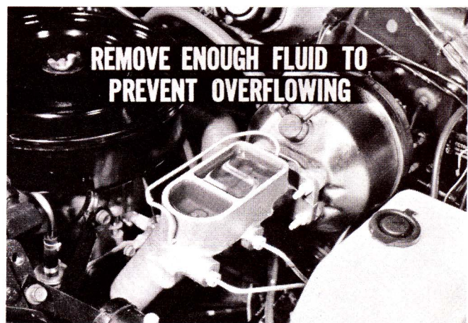
Fig. 2—Moving pistons back raises level
