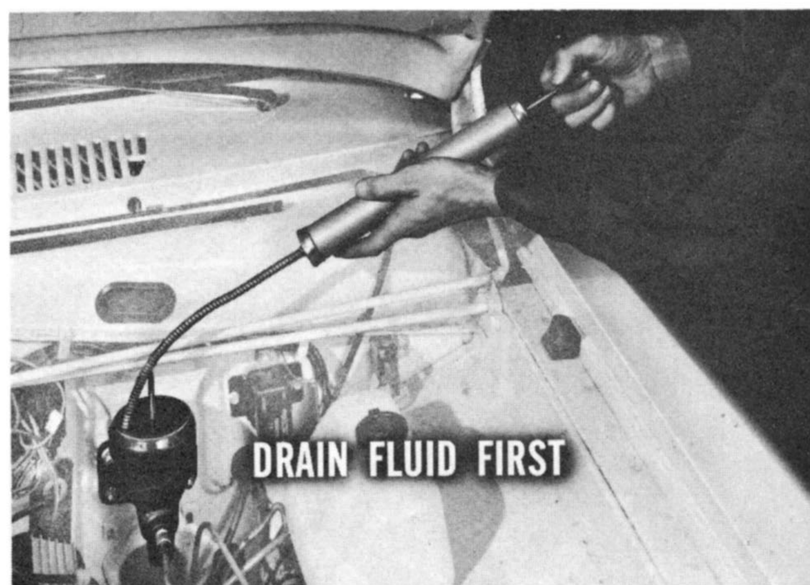
Fig. 22—Make room for fluid in the calipers
