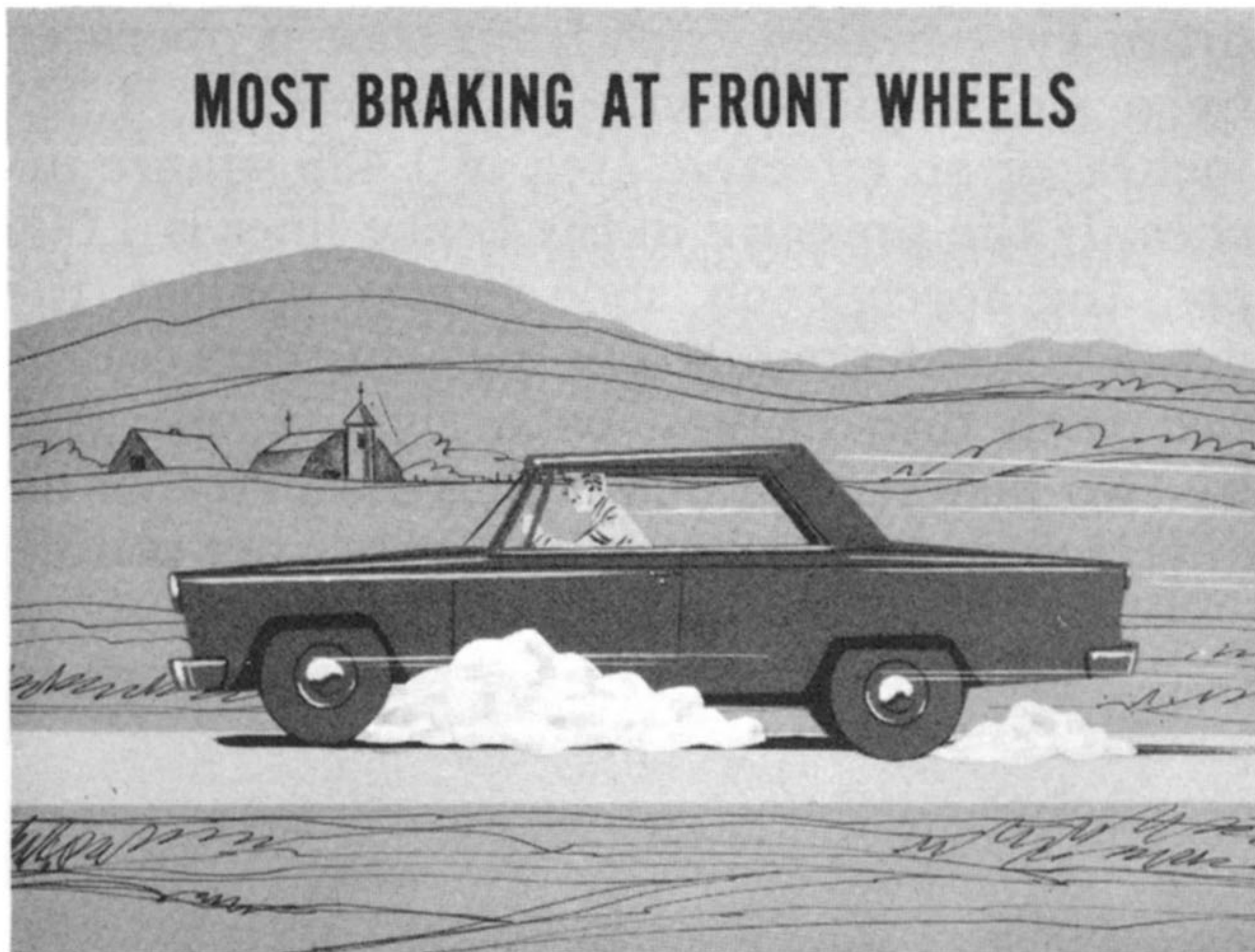
Fig. 2—Most weight is on front wheels
