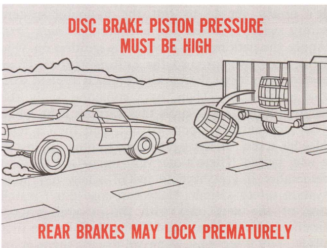
Fig. 20—Tire traction reduced by weight shift
