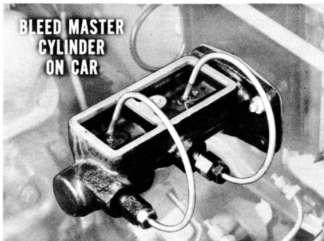
Fig. 33—You can bleed the master cylinder on the car
